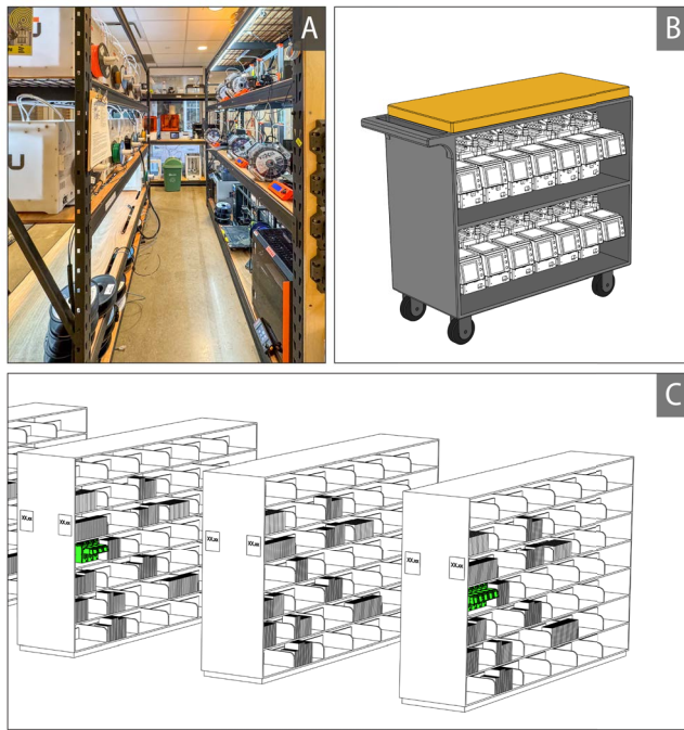
Figure 21: A) A university makerspace print farm that houses ~25 printers. B) A concept for a high-density mobile fabrication cart for education. C) A concept for micro print farms that might be distributed throughout public settings such as libraries.
